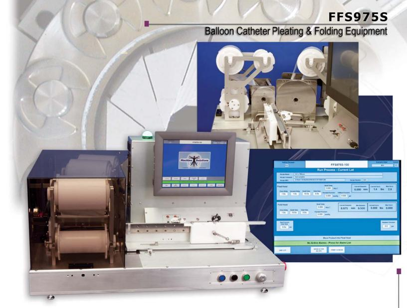
The MSI FFS975S Drug Eluting Balloon Pleating and Folding Equipment is the industry's first and only system specifically designed for processing DEB/DCB products. The FFS975S expands upon industry proven technology with the addition of integrated film, which protects balloon coatings from damage and eliminates the potential for cross contamination that can occur with conventional pleat/fold methods.
