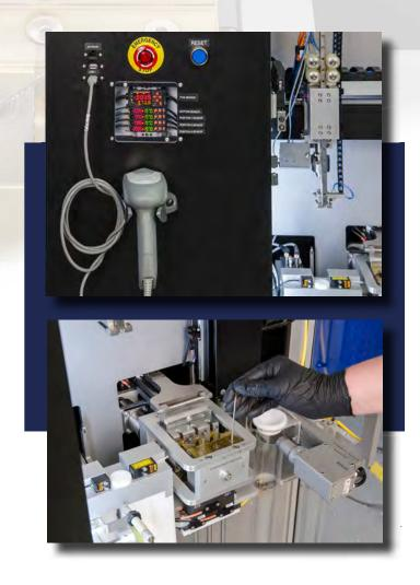
The MSI MS10000 Mandrel Straightening Equipment recycles bent or bowed mandrels through an automated straightening process. The straightener utilizes a pick and place handling system capable of picking a single mandrel from a bin and automatically running it through the straightening process to be placed in the output tube upon completion. The MS1000 has been configured for use with bare and coated stainless steel mandrels of various diameters and lengths with no need for tooling change.
