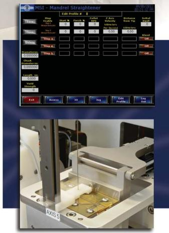
The MSI MS700S Mandrel Straightening Equipment recycles bent or bowed mandrels through an automated straightening process. The straightener utilizes a pick and place handling system capable of picking a single mandrel from a bin and automatically running it through the straightening process to be placed in the output tube upon completion. The MS700S has been configured for use with bare and coated stainless steel mandrels of various diameters and lengths with no need for tooling change.
