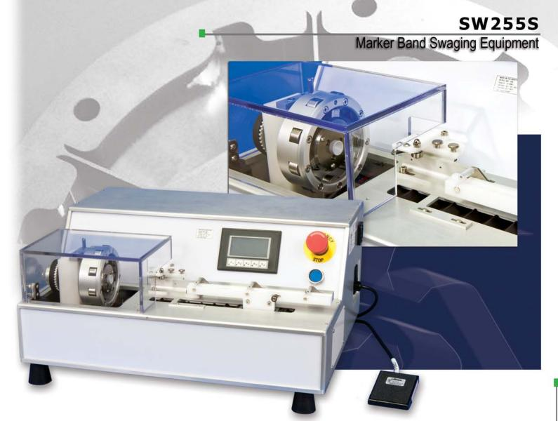
The MSI SW255S integrates our proprietary Element™ swaging technology with an automated handling system and PLC control of traverse speed, traverse distance, swage head rotation speed and the number of swage cycles. The robust Element swaging method is intended for use in swaging a wide range of metal band materials down to a smooth embedded finished diameter.
