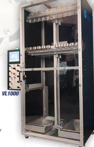
The MSI Vertical Laminator, VL1000 features our Microswirl 360° thermal nozzle that provides superior uniform heating characteristics and minimizes the incidence of hot or cold spots during the shrinking process versus flat or "C" nozzle technologies. We offer machines with four (4) or ten (10) high efficiency heating nozzles which maximize air flow to the product which allows for faster speed and maximum production throughput.
